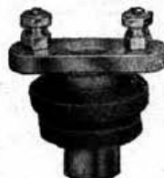
EDDYSTONE All-Wave H.F. Choke. Low loss D.L.-9 former with two section honeycomb wound coils. One screw fixing. Wavering 12.5 to 2,000 metres. Self capacity 2.4 m.mfd. Inductance 17.9 millihenries. D.C. resistance 60 ohms.
