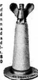
EDDYSTONE Pillar Insulators, made of glazed Frequentite and tested to a breakdown voltage of 30,000. In two types, one having a 2 BA fixing bolt and wing nut, the other a heavy duty plug and socket fitting with soldering tag connections.
