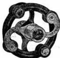
EDDYSTONE Flexible Coupler. Free from backlash but very flexible, this coupler banishes alignment troubles. D.L.-9. H.F. Insulation. For ¼-in. spindles.
