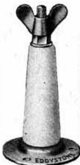
EDDYSTONE Pillar Insulators, made of glazed Frequentite and tested to a breakdown voltage of 30,000. In two types, one having a 2 BA fixing bolt and wing nut, the other a heavy duty plug and socket fitting with soldering tag connections.
